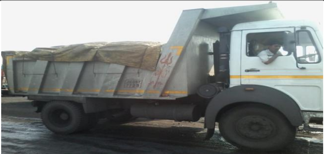
Tarpaulin Cover-Avoid overloading & spillage of valuable coal.
