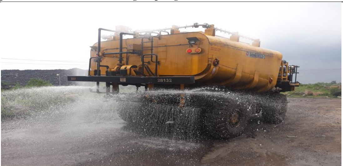
28 KL MIST SPRINKLER AT SDOCM
