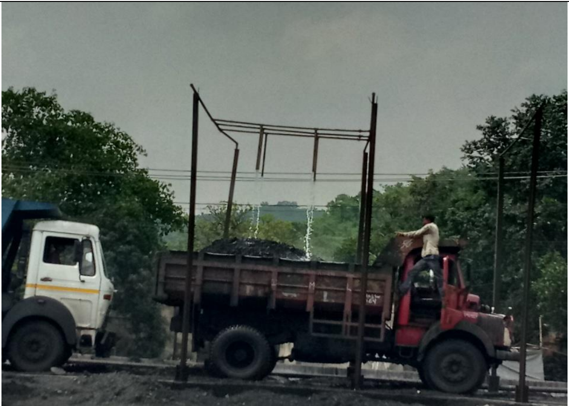
Wetting of Coal before feeding to crusher to suppress dust.
