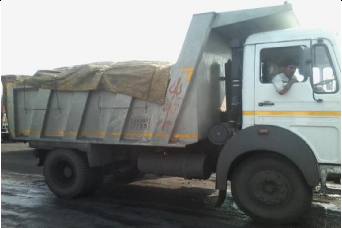
Tarpaulin Cover-Avoid overloading & spillage of valuable coal.
