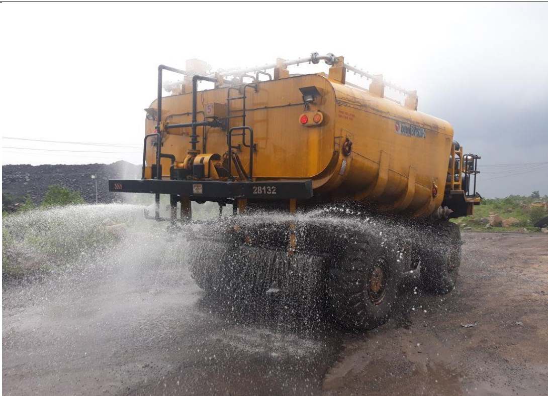
28 KL MIST SPRINKLER AT SDOCM
