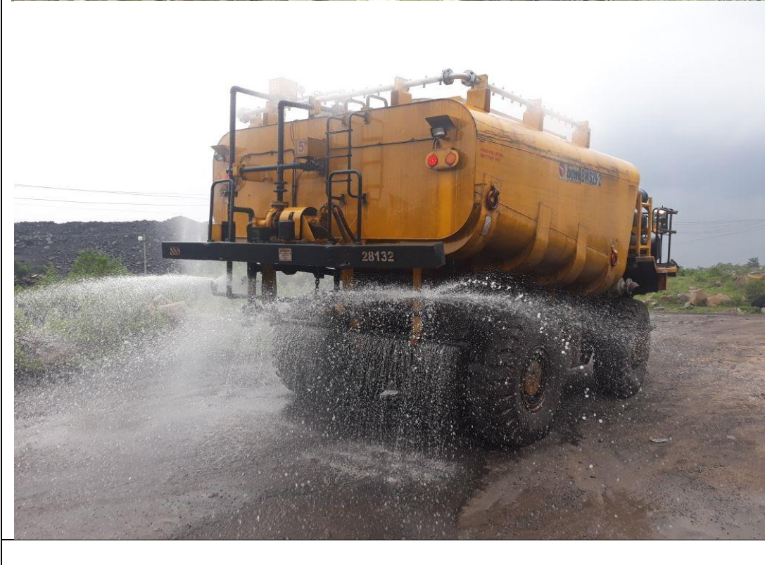
28 KL MIST SPRINKLER AT AMLO OCP
