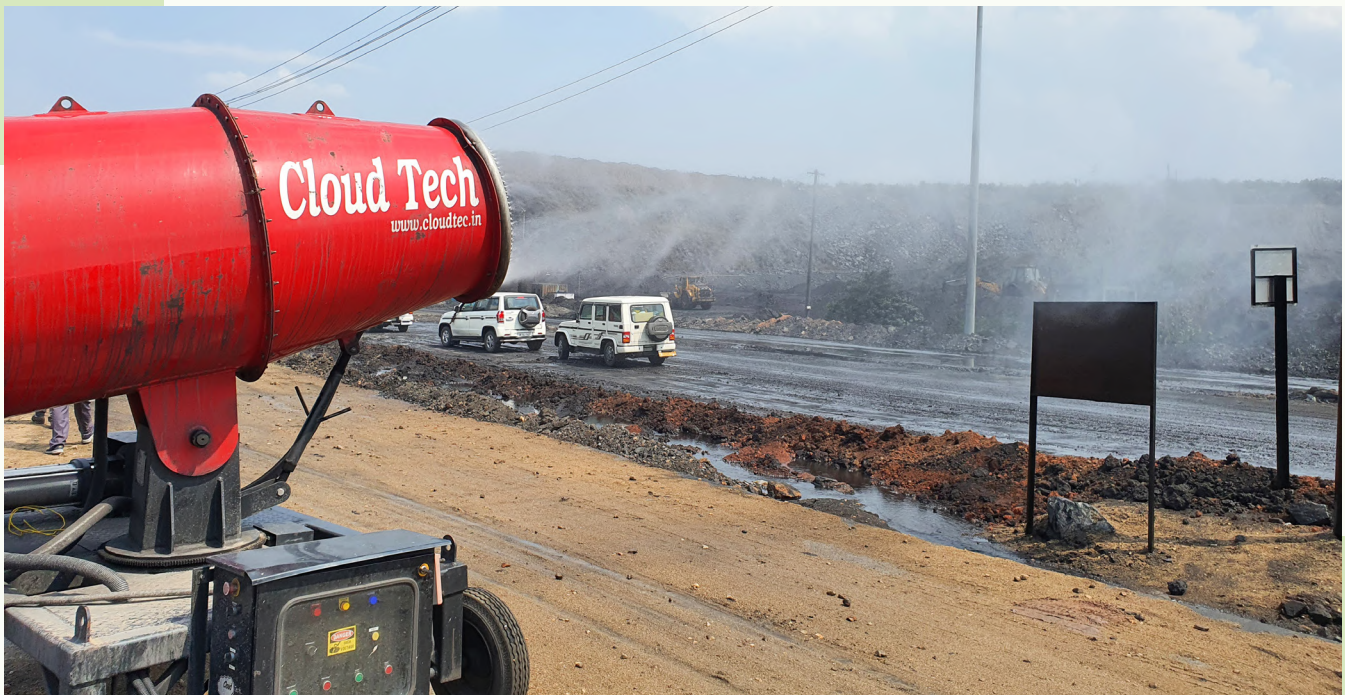
Fog Cannon in operation at Amrapali OCP
