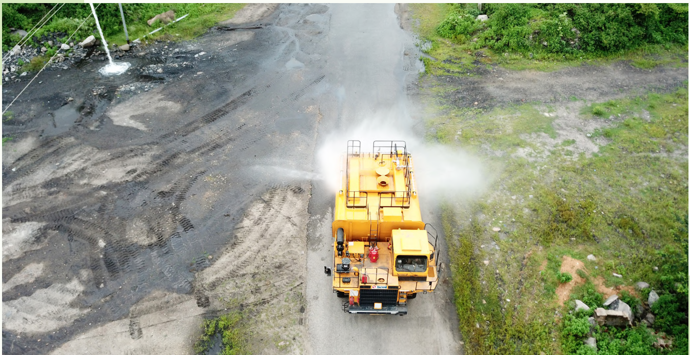
View of Mist Type Water Sprinkler at Rajrappa OCP
